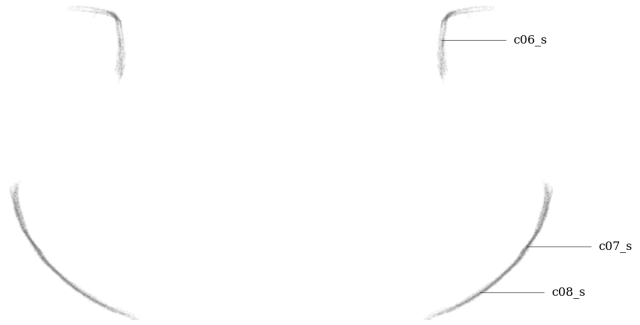
Figure 65: Circularity measurement sample location, separately aligned interior mesh
