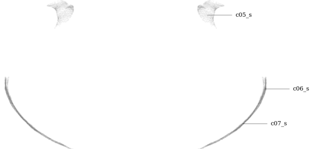
Figure 65: Circularity measurement sample location, separately aligned interior mesh
