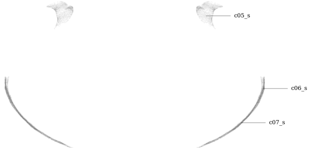
Figure 63: Circularity measurement sample location, separately aligned interior mesh
