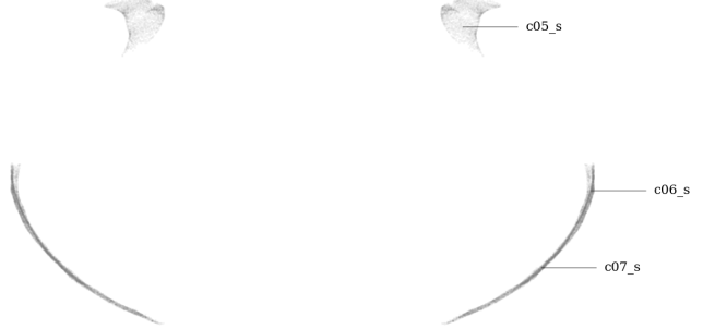
Figure 5: Circularity measurement sample location, separately aligned interior mesh
