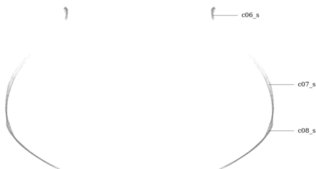
Figure 67: Circularity measurement sample location, separately aligned interior mesh
